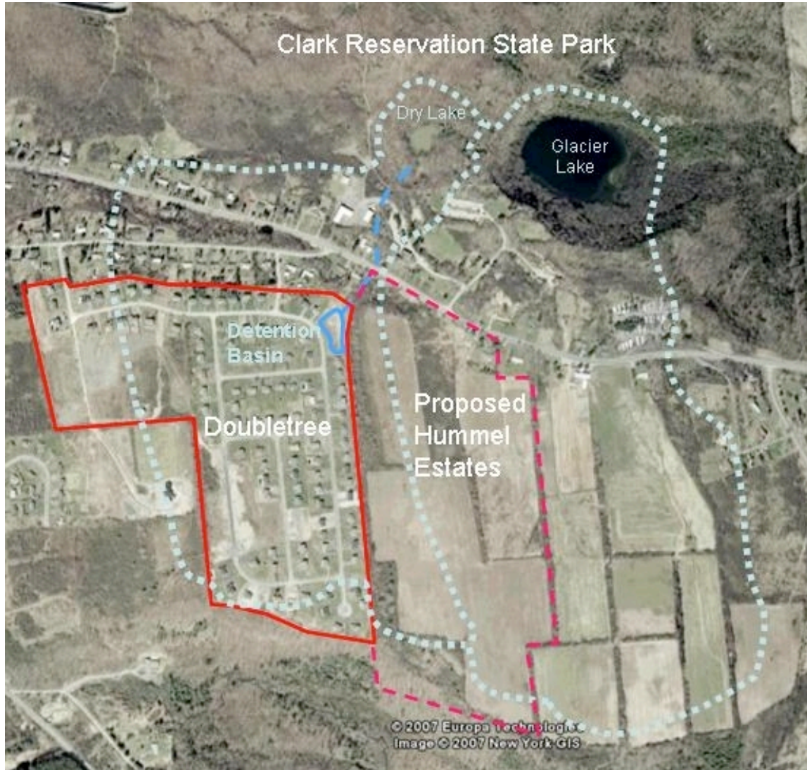
Figure 1: Recent Google Earth view of Dry Lake and Glacier Lake, their watershed areas (dotted light blue), the nearly completed Doubletree residential development (solid red border), and the proposed development Hummel Estates (dotted red border). The detention basin for Doubletree and the intermittent outflow stream that connects to Dry Lake are shown in medium blue.
