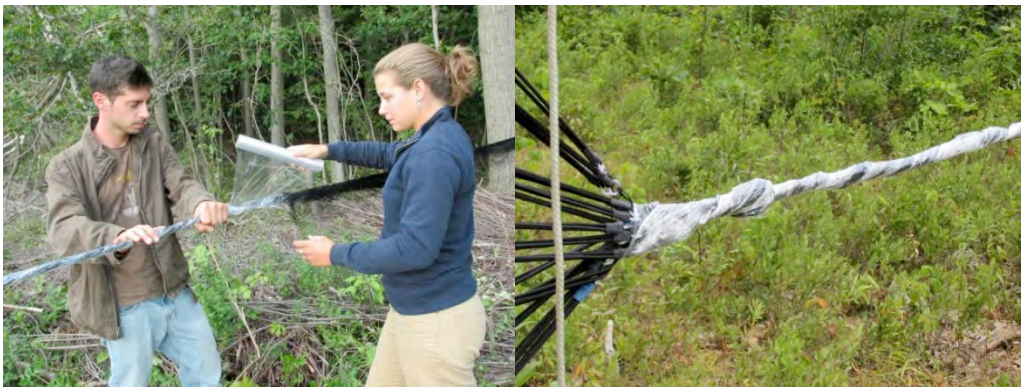
Figure 1. Wrapping a mist net in plastic food wrap.
